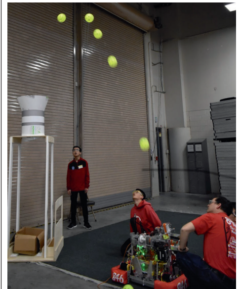
With less aggressive roller speed control and compensating the battery voltage, we now have a consistent shooter!
