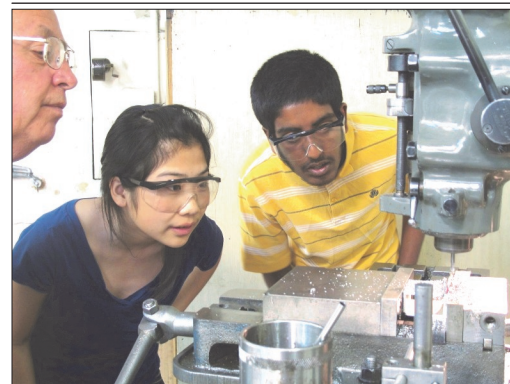
Mr. Lowd, Karena Cai, and Akshara Balachandra face off chassis parts on a mill.
