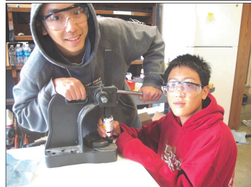
Vincent Yao and Michael Chang press a pinion gear onto a motor.
