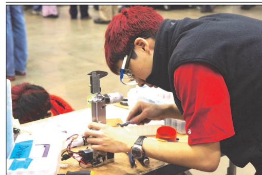
Eric Yeh adjusts the trigger mechanism of the minibot.
