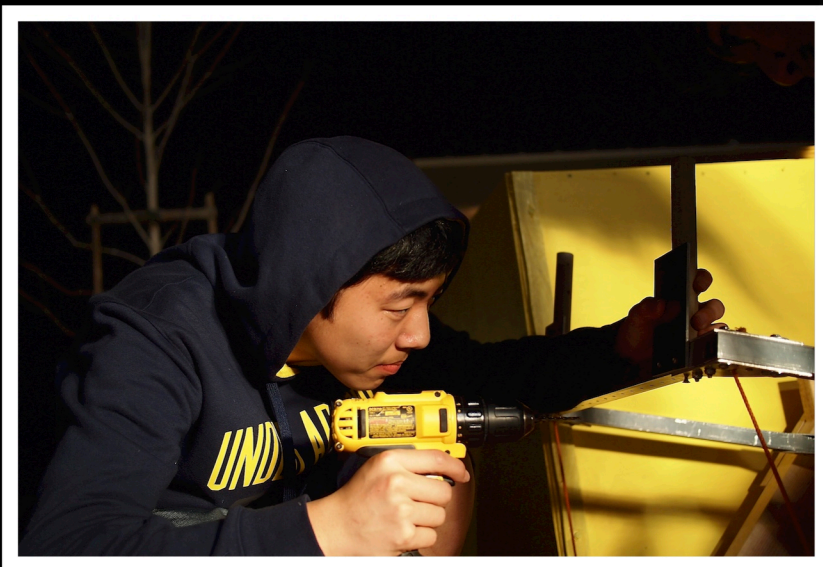
Patrick adjusts the height of the pegs on the shooter prototype to change its launch trajectory.
