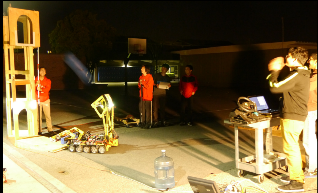
▲ Monkey Python fires a shot during an autonomous run. We practice outdoors at night because the sun interferes with our infrared camera system.
