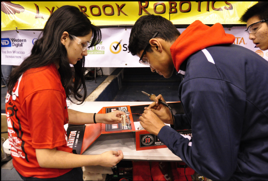
▲ Shalmali Joshi ( mentor ) holds the wire steady as Shikhar Jagadeesh ( junior ) solders the wire to a flashlight for the shooter.
