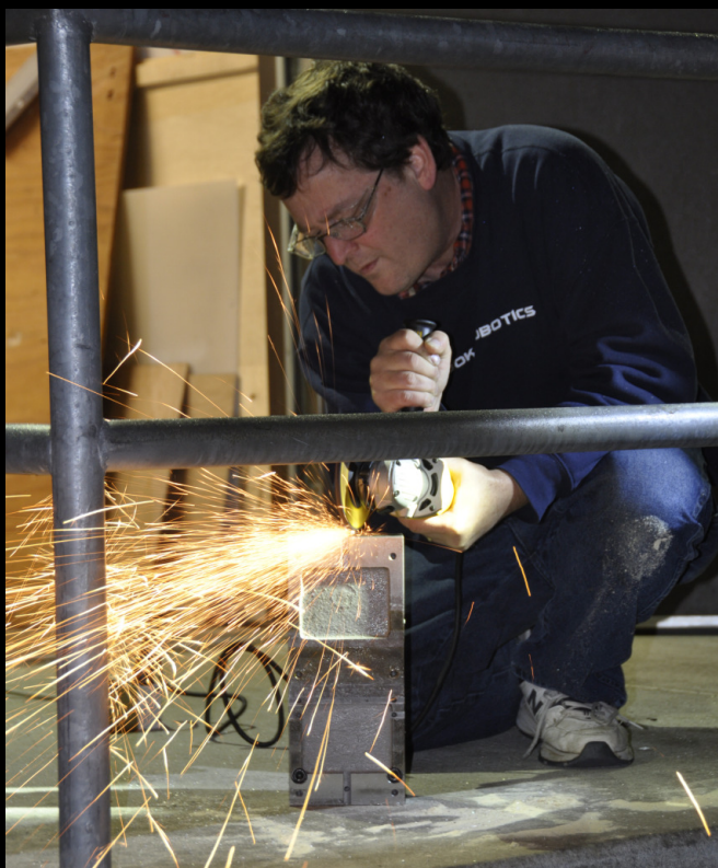
▲ David Giandomenico ( mentor ) makes sparks fly as he repairs the vice on our CNC mill.
