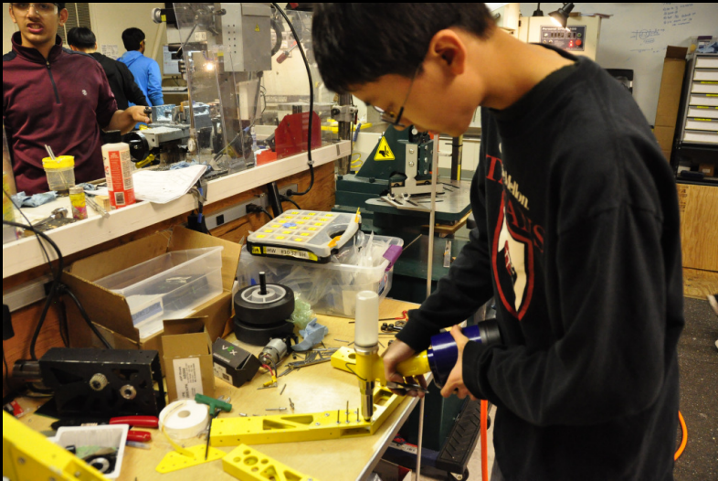
◀ Elton Chang ( sophomore ) carefully rivets pieces of the collector frames together.
